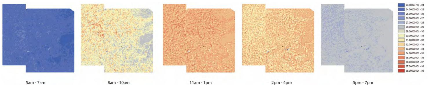
Figure 7. Temperature maps of modelled microclimate data loggers at seven meters height
